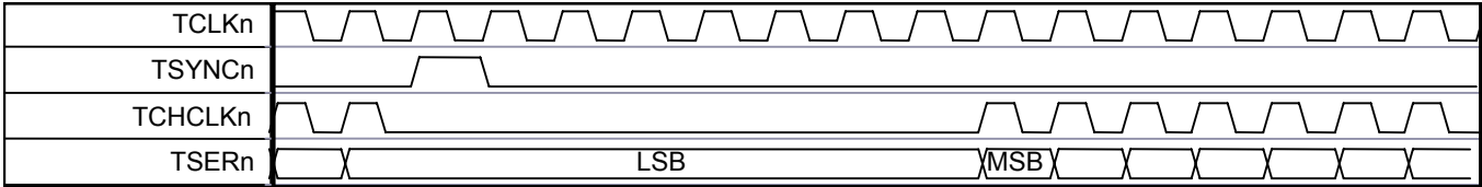
Figure 11-31. E1 Transmit-Side TCHCLKn Gapped Mode During Channel 1
