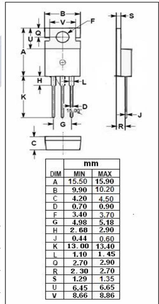
**isc N-Channel MOSFET Transistor**
