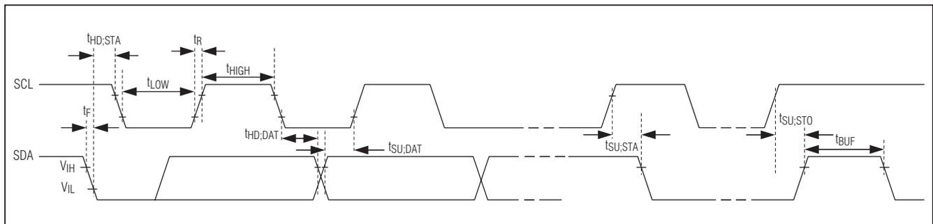
Figure 1. Timing Definitions Used in the Electrical Characteristics
