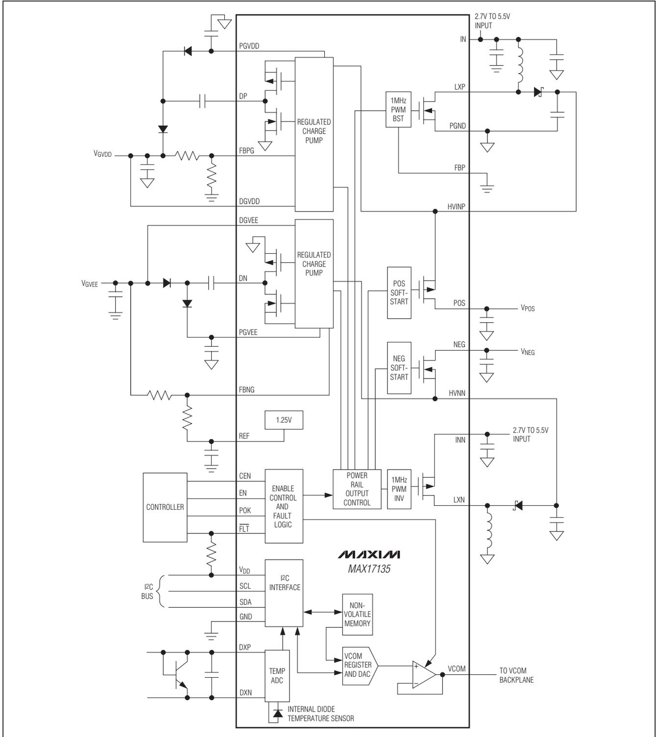
Figure 3. Functional Diagram
