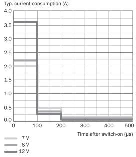
This diagram shows the switch-on current Mechanical self-heating
