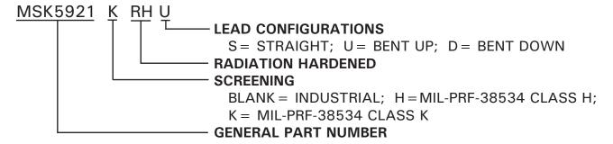
The above example is an adjustable Class K regulator with leads bent up.
