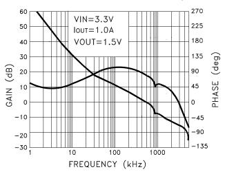
MSK5921RH GAIN AND PHASE vs. FREQUENCY
