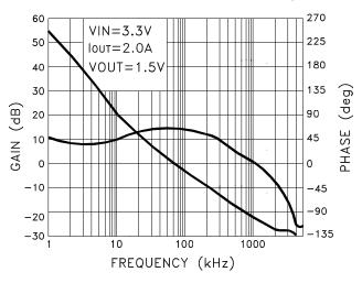
MSK5921RH GAIN AND PHASE vs. FREQUENCY
