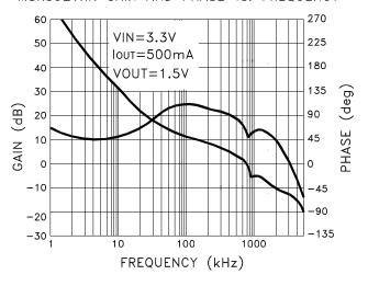
MSK5921RH GAIN AND PHASE vs. FREQUENCY
