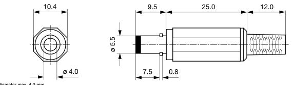
Cable diameter max. 4.0 mm
