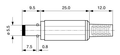
Cable diameter max. 4.0 mm
