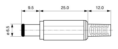
Cable diameter max. 4.0 mm
