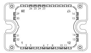
All multiple inputs and outputs must be shorted together 10/11; 23/24; 2/3; ...
