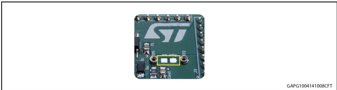
Figure 5: Pads for soldering SMD resistor
