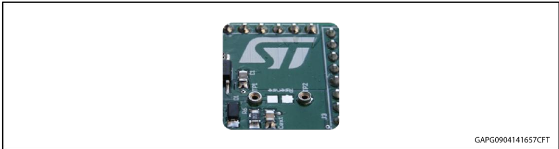
Figure 4: Mounting through-hole sense resistor
