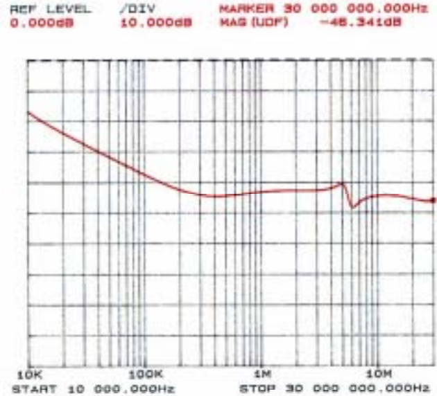
Figure 2: Typical differential-mode insertion loss in a 50 circuit
