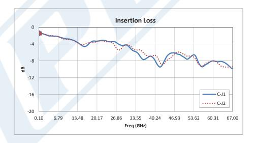
Click the following link (or enter part number in "SEARCH" on website) to obtain additional part information including price, inventory and certifications: Absorptive SPDT PIN Diode Switch Operating From 100 MHz to 67 GHz Up to +27 dBm and 1.85mm PE71S2026
