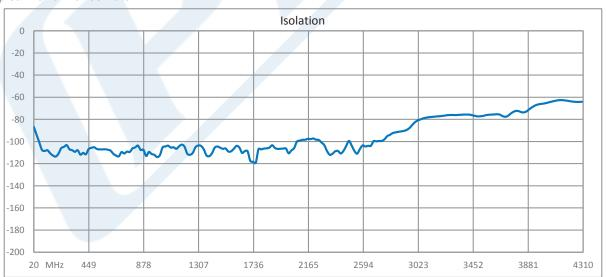
Click the following link (or enter part number in "SEARCH" on website) to obtain additional part information including price, inventory and certifications: Absorptive SPDT PIN Diode Switch Operating From 20 MHz to 4.3 GHz Up to 1 Watt (+30 dBm) and SMA PE71S2035
