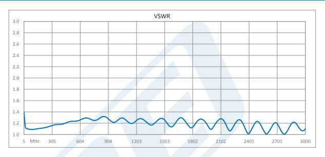
Absorptive SPDT PIN Diode Switch Operating From 5 MHz to 3 GHz Up to 1 Watt (+30 dBm) and SMA from Pasternack Enterprises has same day shipment for domestic and International orders. Our RF, microwave and millimeter wave products maintain a 99.4% availability and are part of the broadest selection in the industry.
