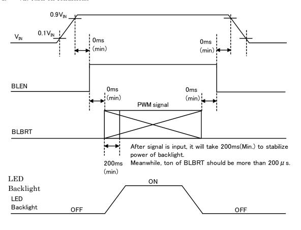
2)  $V_{IN} = 12V$ , Temp. = 25 ,  $D_{PWM} = 100\%$
