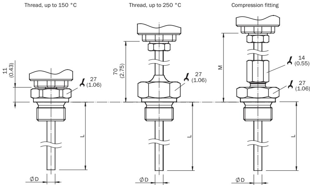
Process connections, conical threads
