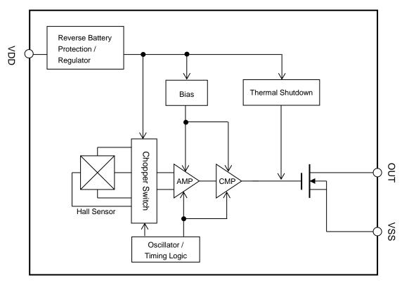
Figure 1. EM6011 Block Diagram
