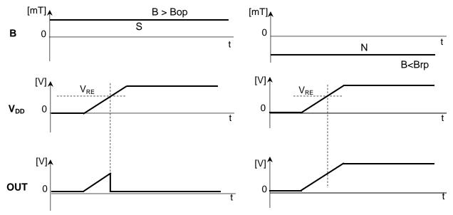
Figure 4. Output waveform in power on
