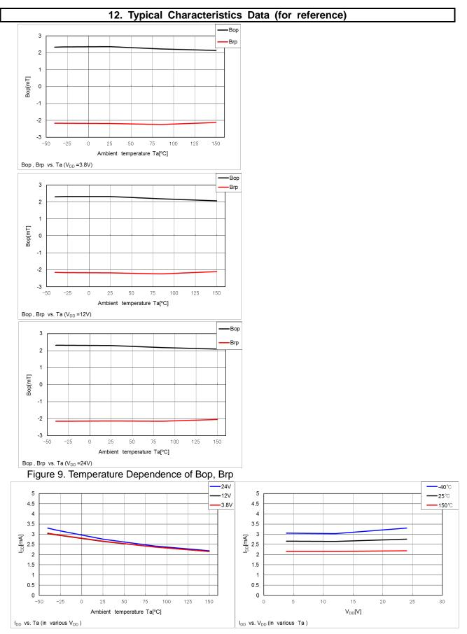
Figure 10. Temperature Dependence of Current Consumption
