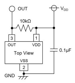
Figure 8. Recommended External Circuit
