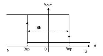
Figure 7. Switching behavior of OUT signal when magnetic field is applied
