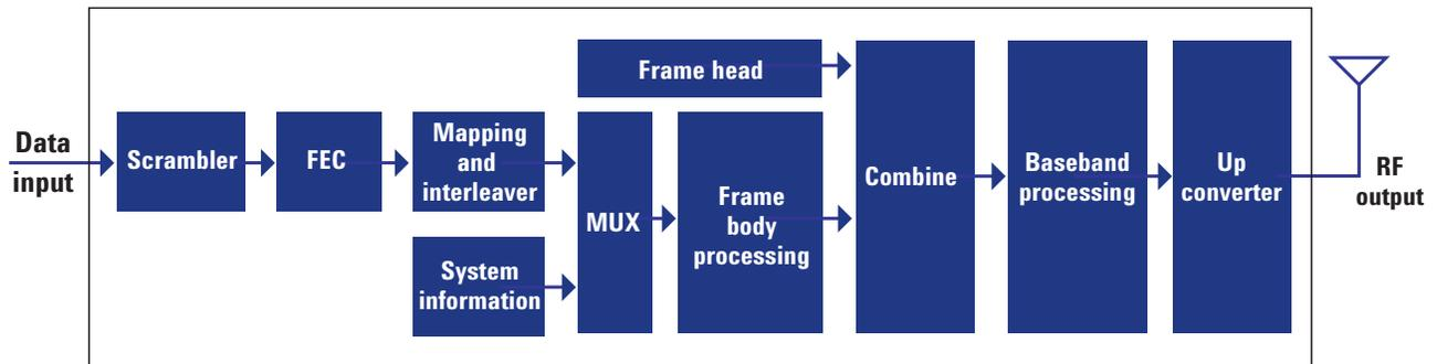
Figure 1. Block diagram of DTMB (CTTB) system
