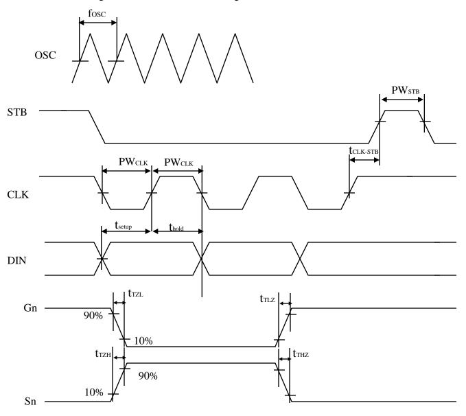
PW <sub>CLK</sub> (Clock Pulse Width)  $\geq$ 400ns t setup (Data Setup Time)  $\geq$  100ns t <sub>CLK-STB</sub> (Clock - Strobe Time)  $\geq$  1 $\mu$ S t <sub>TZH</sub> (Rise Time)  $\leq$  1 $\mu$ S t <sub>TZL</sub> <1 $\mu$ S
