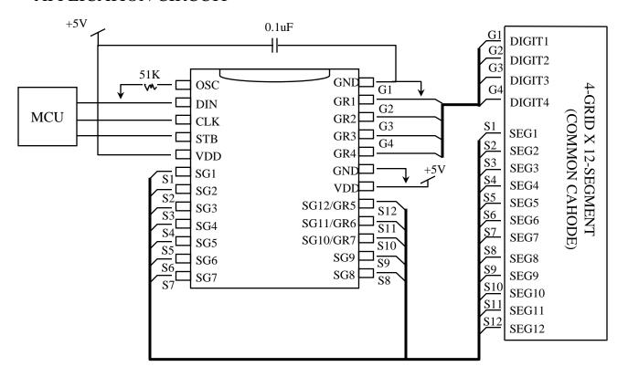
Note: The capacitor (0.1uF) connected between the GND and VDD Pins must be located as near as possible to the IK2107 chip.
