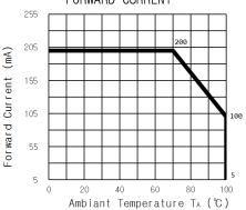
Fig.5 FORWARD CURRENT DERATING CURVE
