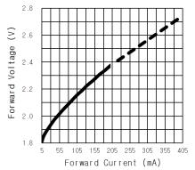
Fig. 3 FORWARD VOLTAGE V.S. FORWARD CURRENT
