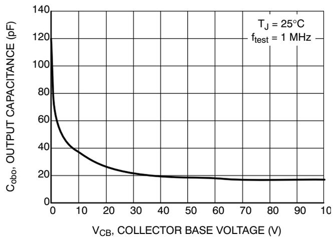
Figure 11. Output Capacitance
