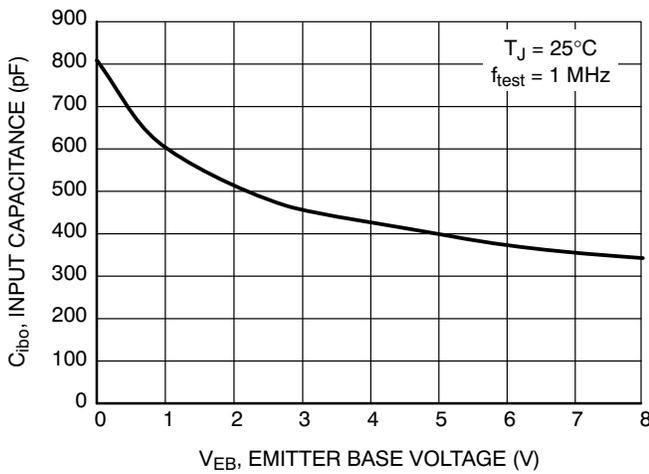
Figure 10. Input Capacitance
