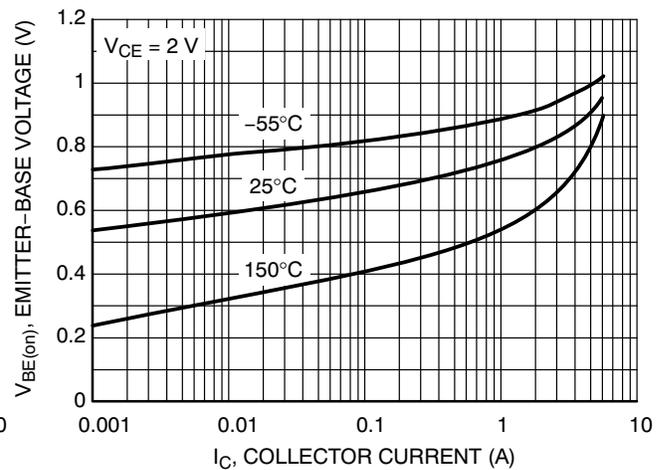
Figure 7.  $V_{BE(on)}$  Voltage
