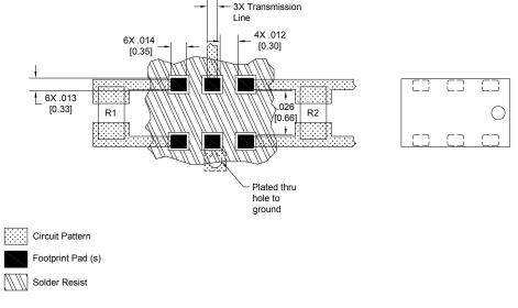
Dimensions are in Inches [Millimeters] Mounting Footprint
