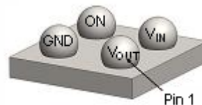
Figure 4. WLCSP Bumps Facing Up (Bottom View)
