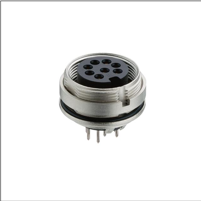
SWUM™ chassis socket acc. to IEC 61076-2-106 and AISG specification, IP 68/67, with threaded joint, for printed circuit boards, manual soldering, for back side mounting
