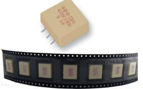
The CB style capstick capacitor is constructed non-inductively with metallized polyester dielectric. The low inductance and low ESR construction makes it ideal for high frequency switching power supplies. CB type capacitors can be used with pick and place assembly and the -FS parts are fully RoHS compliant and capable of high temperature lead free soldering.
