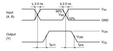
Figure 2 t<sub>pLH</sub>, t<sub>pHL</sub>
