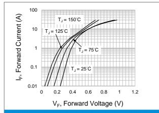
Fig.4 Typical Forward Characteristics
