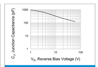
**Fig.2 Typical Junction Capacitance**
