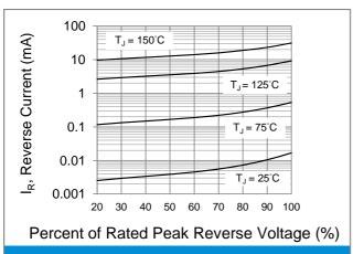
**Fig.3 Typical Reverse Characteristics**
