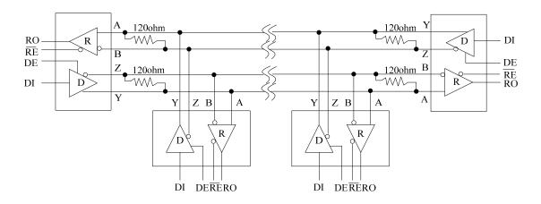
Figure 2: Typical Full-Duplex RS-422 Network
