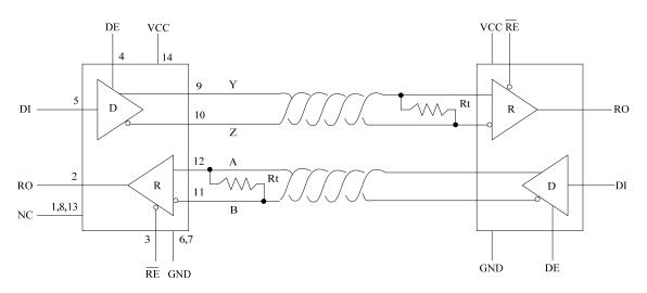
Figure 1: UM491 pin configuration and typical full-duplex operating circuit
