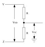
Figure 3. Driver DC Test Load
