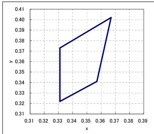
Note 1) The tolerance of measurement at our tester is  $V_F \pm 3\%$  ,  $\Phi_v \pm 10\%$  , Chromaticity(x,y) $\pm 0.01$ .
