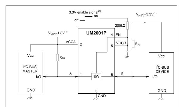
(1) In the Enabled mode, the applied enable voltage  $V_{I(EN)}$  and the applied voltage at  $V_{CCA}$  should be such that  $V_{CCB}$  is at least 1 V higher than  $V_{CCA}$  for best translator operation.
