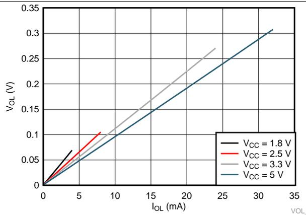
Figure 1. Typical  $I_{OL}$  vs.  $V_{OL}$  ( $T_A = 25^\circ\text{C}$ )
