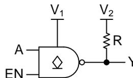
**Figure 6. Gated Voltage Translating Inverter Schematic Using SN74LVC1G38**
