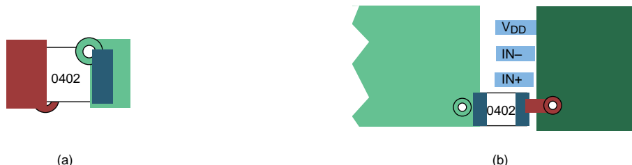
Figure 15. Typical Decoupling Capacitor Layouts
