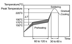
[Allowable Reflow Soldering Temperature and Time]
