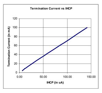
The termination current is always roughly 10% of the maximum charge current set by the HCP resistor.
