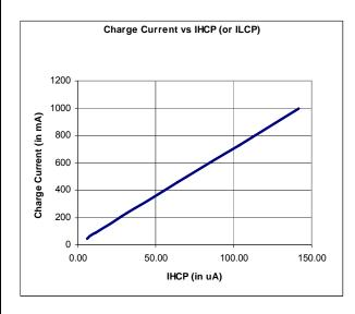
Using the table below it can be seen that for a programming current value of  $11.4\mu A$ , the corresponding maximum charge current is 92mA.
