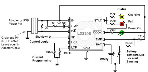
**Figure 1** – Typical Application – 1A or 500mA maximum charge currents with three indicators and battery temperature lockout. A grounded spare pin in the USB power cable can be used to sense when the 500mA USB current power source is being used.
