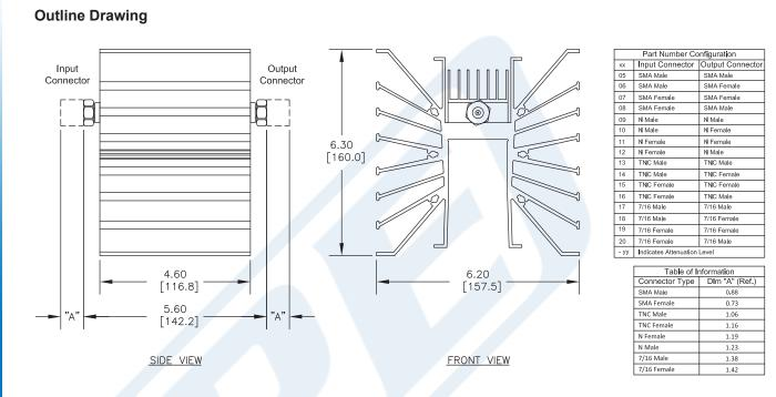
50 dB Fixed Attenuator, SMA Female To SMA Female Directional Black Aluminum Heatsink Body Rated To 300 Watts Up To 3 GHz from Pasternack Enterprises has same day shipment for domestic and International orders. Our RF, microwave and millimeter wave products maintain a 99% availability and are part of the broadest selection in the industry.
