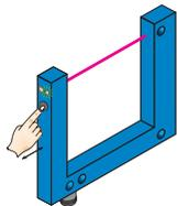
Press the teach-in button for 3 - 20 s. With the pushbutton pressed down, move several objects with carrier material (label objects to be detected) through the sensor. The yellow LED flashes at 3 Hz during the teach-in procedure. Recommendation: Move at least 3 objects through the sensor.
