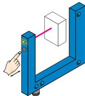
Release the teach-in button for < 20 s. If teach-in is successful, the function indicator (yellow LED) directly indicates the output state of the sensor. The switching threshold is now optimally set between background and object. The best possible operational safety is provided.
