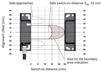
If the actuator moves laterally in relation to the surface of the sensor, a minimum distance of 9 mm must be maintained. This distance will prevent premature triggering due to the side approach areas.
