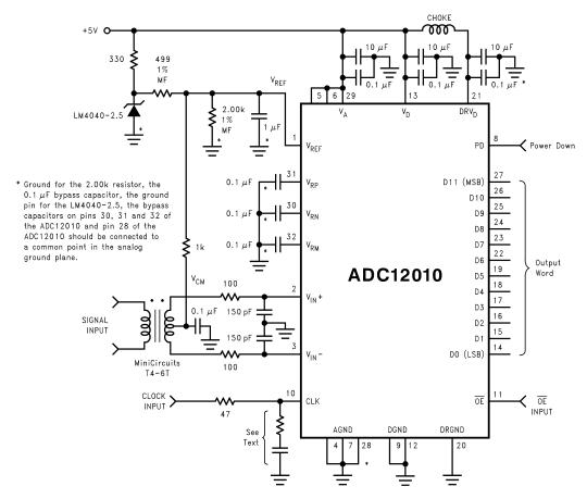
Figure 39. Driving the Signal Inputs with a Transformer
