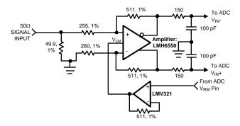
Figure 38. Differential Drive Circuit of Figure 37
