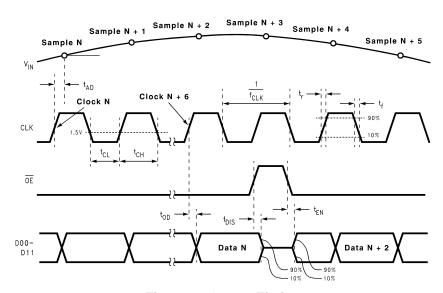
Figure 1. Output Timing
