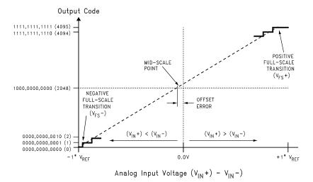
Figure 2. Transfer Characteristic
