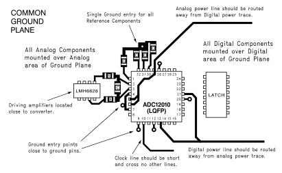
Figure 40. Example of a Suitable Layout
