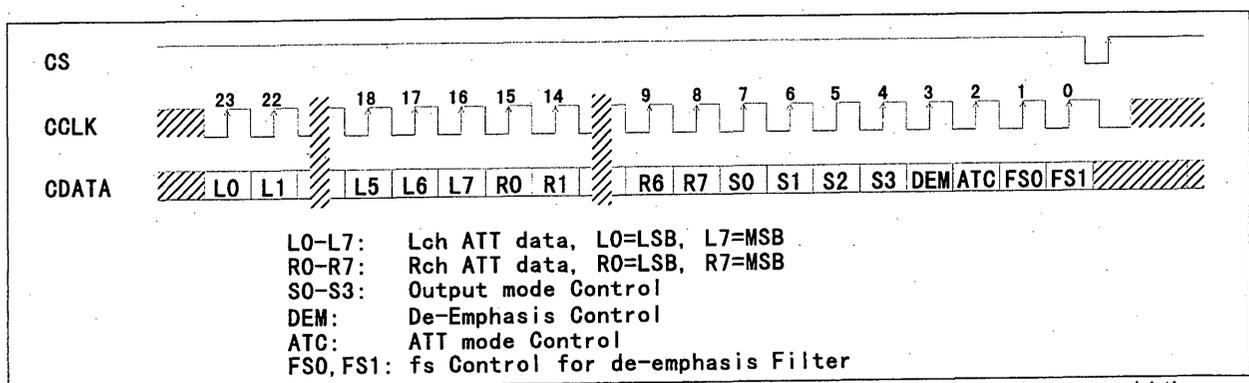
note: CCLK should be held "H" or "L" except writing to ATT & mode registers in order to avoid the performance degradation.
