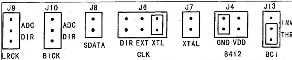
Figure 3. Jumper Set-up(ROM)
