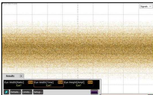
Figure 27. TL = 7-Meter 30-AWG 100 Ω Twin-Axial Cable, No Repeater, 10.3125 Gbps
