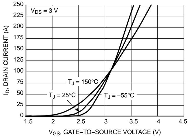
Figure 2. Transfer Characteristics
