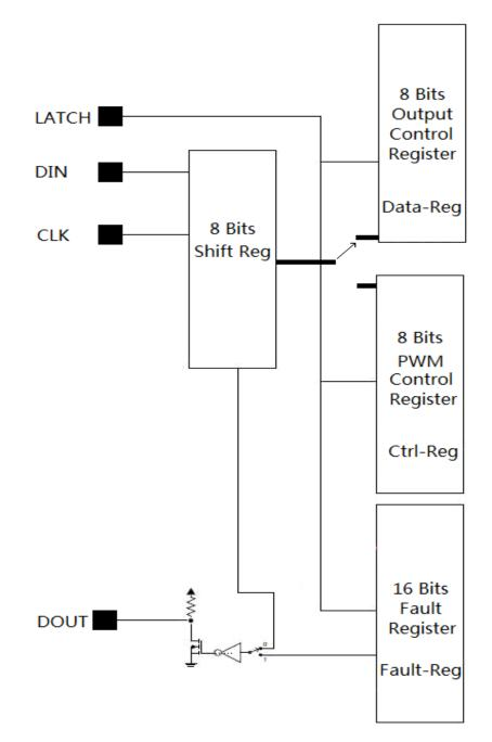
In default condition, 8 Bit shift register data moves into output control register DATA-REG
