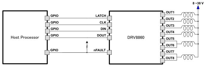
Example Configuration 2: DRV8860 Drives Multiple Low Side Loads With Parallel Configuration
