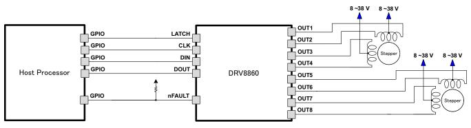
Example Configuration 3: DRV8860 Drives Two Unipolar Stepper Motors
