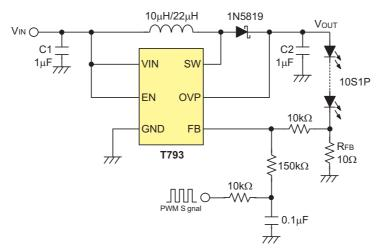
Figure 11. Application Circuit for Dimming Control Using a Filtered PWM Signal
