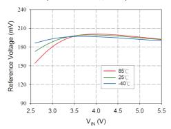
Figure 4. Reference Voltage vs. Input Voltage (10S1P)
