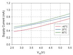
Figure 8. Supply Current vs. Input Voltage  $(V_{FB}=GND)$
