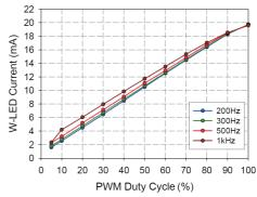
Figure 6. LED Current vs. PWM Duty Cycle (9S1P)
