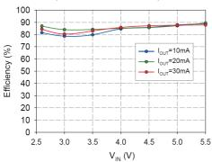
Figure 3. Efficiency vs. Input Voltage (Boost Mode V<sub>OUT</sub>=33V)
