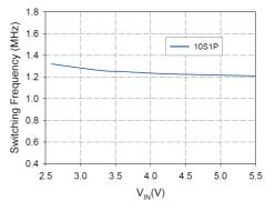
Figure 7. Switching Frequency vs. Input Voltage
