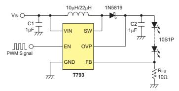
Figure 9. Application Circuits for Driving 10S1P WLEDs
