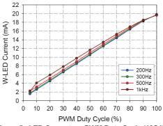
Figure 5. LED Current vs. PWM Duty Cycle (10S1P)
