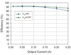
Figure 2. Efficiency vs. Input Voltage (Boost Mode V<sub>OUT</sub>=10V)
