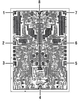
$\begin{array}{c} 117 \text{mils} \times 82 \text{mils}, \\ 12 \text{mils thick}. \\ \text{Backside (substrate) is an alloyed gold layer.} \\ \text{Connect backside to V}^+. \end{array}$
