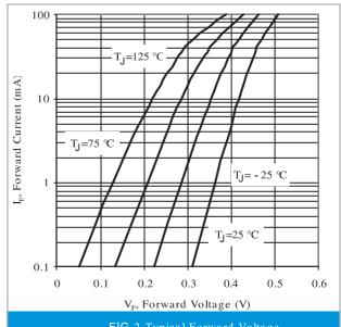
FIG.2-Typical Forward Voltage
