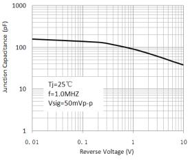
Figure 4. Typical Junction Capacitance
