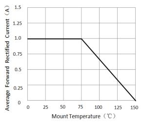
Figure 1.Forward Current Derating Curve
