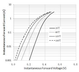
Figure 2. Typical Instantaneous Forward Characteristics
