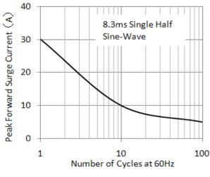
Figure 5.Maximum Non-Repetitive Peak Forward Surge Current
