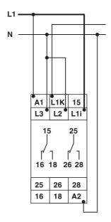
1  $\sim$  230 V measuring range, without error memory, 230 V AC supply voltage,  $\rm I_N < 10~A$
