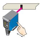
When detecting the contrast or color to be detected, "1st" flashes.
