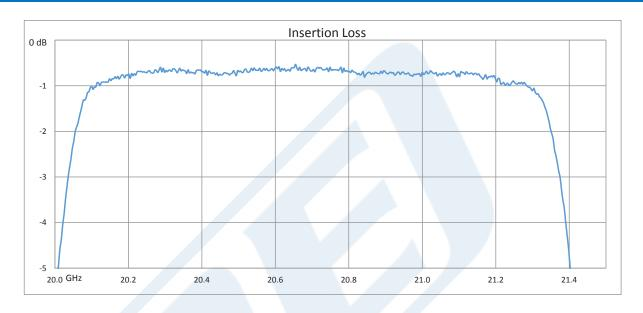
Click the following link (or enter part number in "SEARCH" on website) to obtain additional part information including price, inventory and certifications: 6 Section Bandpass Filter With SMA Female Connectors Operating From 20.2 GHz to 21.2 GHz With a 1,000 MHz Passband PE87FL1011
