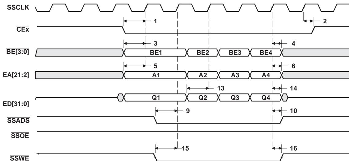
Figure 18. SBSRAM Write Timing (1/2 Rate SSCLK)
