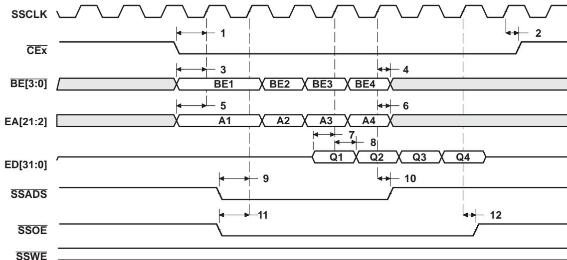
Figure 17. SBSRAM Read Timing (1/2 Rate SSCLK)
