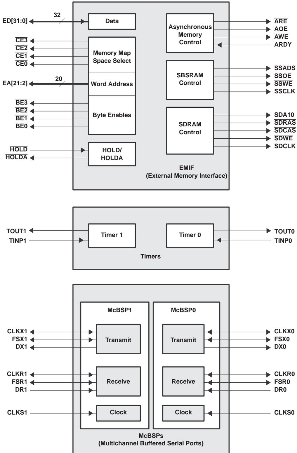
Figure 4. Peripheral Signals
