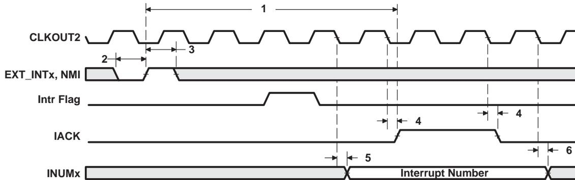
Figure 27. Interrupt Timing
