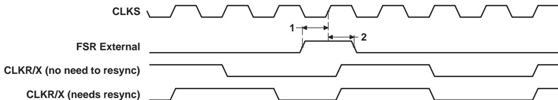
**Figure 33. FSR Timing When GSYNC = 1**
